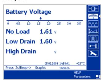
Low drain batteries are automatically tested with a load resistance matching the battery and high drain batteries are manually tested by pressing a button.
