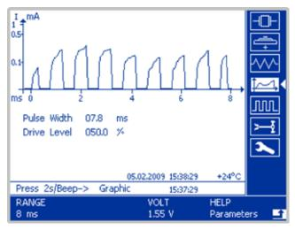
The shape of the motor pulse current is shown as a curve. The pulse shape is an important criterion about the good operation of the watch. Errors in the mechanical part of the watch can be determined by comparative measurements with a good watch of the same type. The pulse width and the chopping level are displayed numerically.
