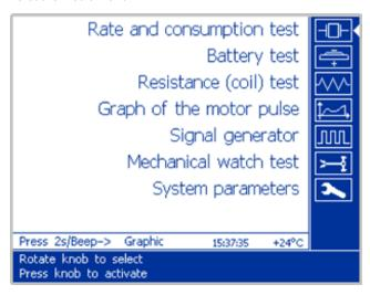
The operation is simple and easy to understand. Ordinary standard measurements can be largely automated. The instrument determines the associated parameters. For more advanced users, measuring parameters can also be manually selected according to requirements. The results, menus and parameters appear on the ¼ VGA LCD graphic display.
