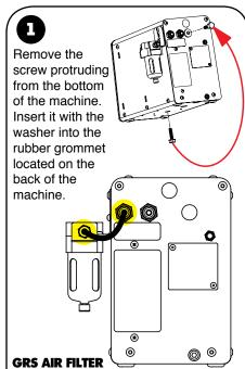
Connect the air filter to the GraverMax G8 by loosening the side cover screw and sliding the bracket onto the screw. Re-tighten screw.
