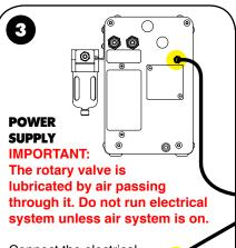
power cord into the box. Plug the converter cord into the jack on the back of the machine.
