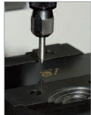
Flachgravur – Fräser Flat engraving – milling cutter
