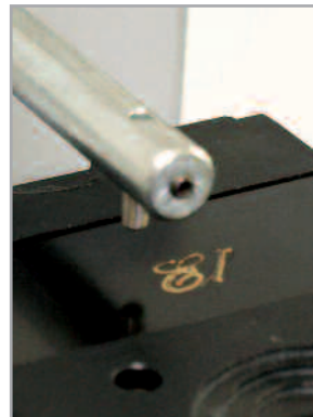
Flachgravur – Diamant Flat engraving – diamond
