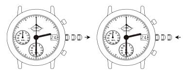
3.Pull out the crown to the second click when the second hand is at the 12 o'clock position. It will stop on the spot and advance the hour and minute hands by turning the crown. (Check that AM/PM is set correctly.)
