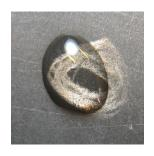
After a few seconds the stroke is coated by one clearly visible, white covering (turbidity).
