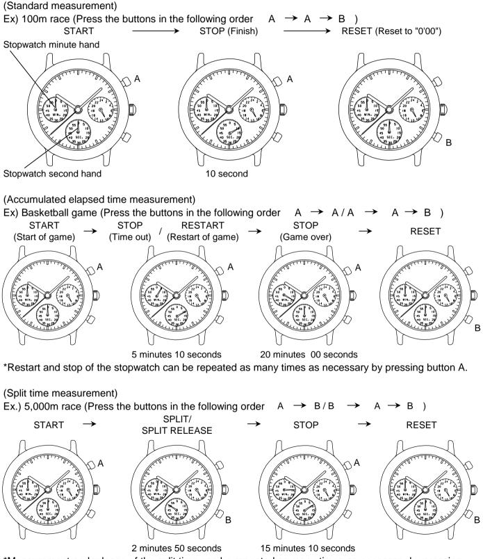
\*Measurement and release of the split time can be repeated as many times as necessary by pressing button B.
