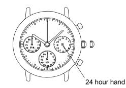
2.Turn the crown to set the hour, minute and 24 hour hands to the desired time.As the hour hand moves, the
