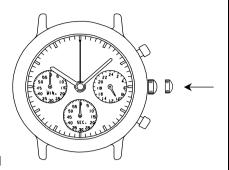
3.Push the crown back in to the normal position in accordance with a time signal.
