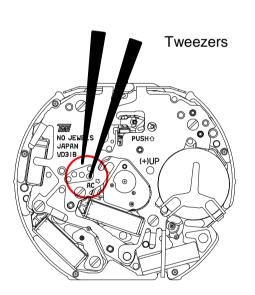
(3) When the battery replaced with a new one, the time information stored in the built-in IC and the time indicated by the dual time of 24 hour hand do not correspond with each other. Reset the dual time of 24 hour hand to "0" position following the procedure below. If the dual time of 24 hour hand should move improperly, also follow the same procedure.
