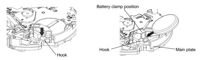
(2) After the battery is replaced with a new one or after the battery is reinstalled following the repairing procedures, Be sure to touch the short-circuit the AC terminal of circuit block and the switch spring with conductive tweezers to reset the circuit as illustrated at right.
