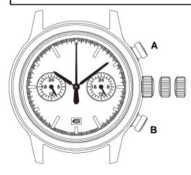
1.Pull out the crown when the second hand is at the 12 o'clock position.[ Crown position ]
