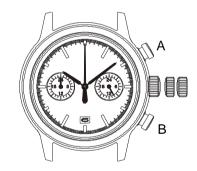
3.Press button A or B to reset the dual time of 24 hour hand to "0" position.
