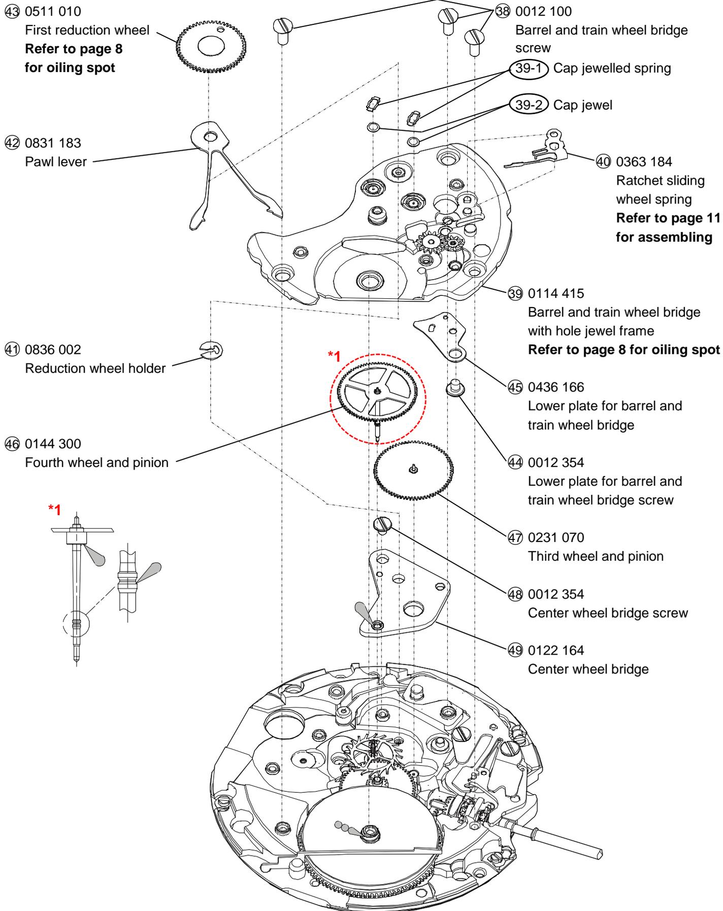
Disassembling procedures Figs.
