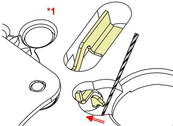
Remove the hook of the ratchet sliding wheel spring from barrel and train wheel bridge with hole jewel frame.
