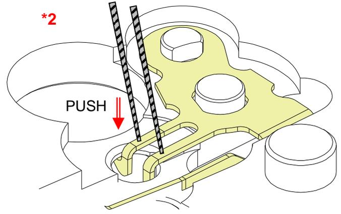
The hooks of ratchet sliding wheel spring are hung up on barrel and train wheel bridge with hole jewel frame.
