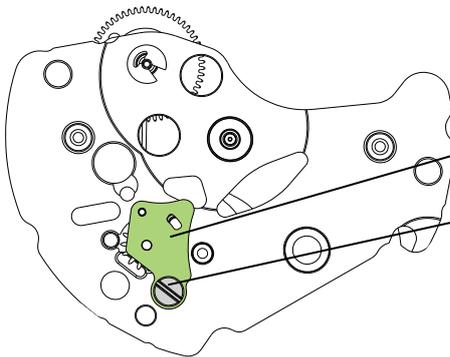
④5 Lower plate for barrel and train wheel bridge
