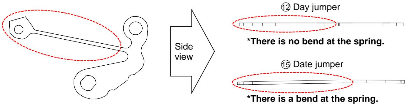
4.Disassembling / assembling of the First reduction wheel
