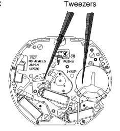
2) When the battery replaced with a new one, the time information stored in the built-in IC and the time indicated by the stopwatch hands do not correspond with each other. Reset the stopwatch hands to "0" position following the procedure below. If the stopwatch hands should move improperly, also follow the same procedure.
