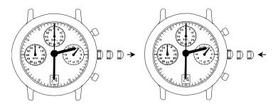
3.Pull out the crown to the second click when the second hand is at the 12 o'clock position. It will stop on the spot and advance the hour and minute hands by turning the crown. (Check that AM/PM is set correctly.)
