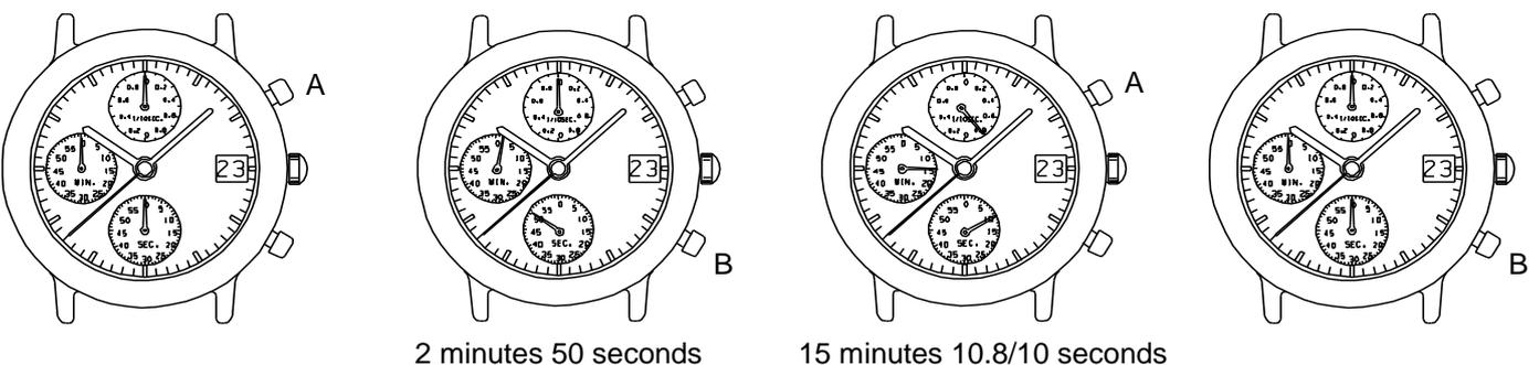
\*Measurement and release of the split time can be repeated as many times as necessary by pressing button B.
