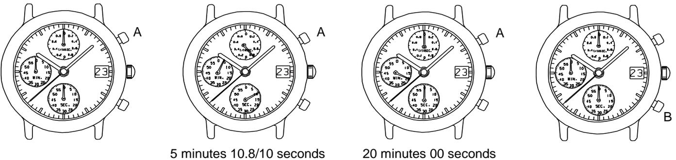
\*Restart and stop of the stopwatch can be repeated as many times as necessary by pressing button A.
